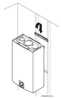
Fig. 24 Mounting the heater
